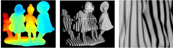
**Figure 7:** Simulating illumination defocus effect of the projector. (left) Depth of the scene as seen by the projector. The focal plane is placed halfway between the maximum and minimum depth; (middle) final scene as seen by the camera; (right) details of the rectangle highlighted in the middle image.
